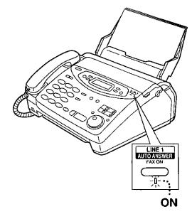
If you have a telephone line just for receiving faxes, we recommend the following setup.
